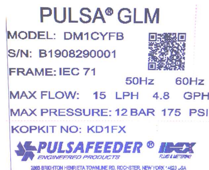
Figure 19: PULSA GLM ® Nameplate
